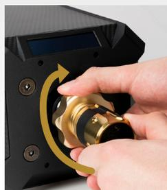
**⚠ IMPORTANT: DO NOT** pull out the steering axle forcefully by hand other wise it is possible to tear off the cables inside the steering axle.
