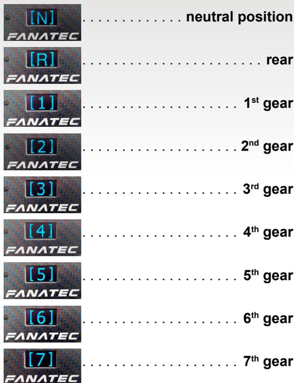
If your shifter has no 7th gear just acknowledge it by pressing the **FunkySwitch™** when the shifter lever is physically in position of 6th gear. After all gears are calibrated the OLED display shows SET 1 and the shifter is ready for use.
