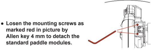
marked red in picture by Allen key 4 mm to detach the standard paddle modules.
