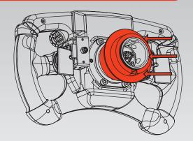
• Pull off the steering wheel from the wheel base axle.
