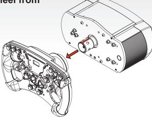
• Press or "pinch" and hold the Quick Release mechanism.
