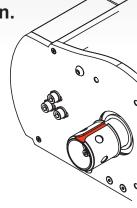
• Press togther or "pinch" and hold Quick Release mechanism.
