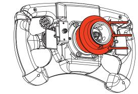
• Slide the steering wheel onto the wheel base axle up to the mechanical limit.
