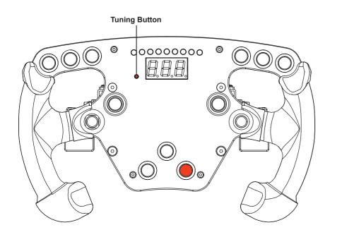
To enter tuning menu, press tuning button. To navigate inside the menu, use the right FunkySwitch<sup>™</sup>. Press it up or down to access 5 setups. Press FunkySwitch<sup>™</sup> right or left to go through the options and turn the FunkySwitch<sup>™</sup> to change option values.
