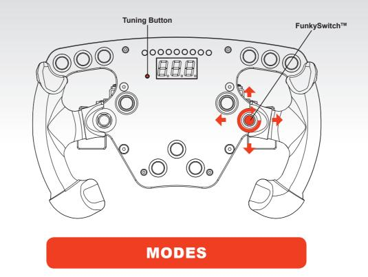
To switch between modes simultaneously press and hold the two buttons highlighted below, for one second. The wheel base LED indicates the active mode:
