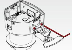
Connect the ClubSport Magnetic Paddle Module cables to the highlighted sockets.
