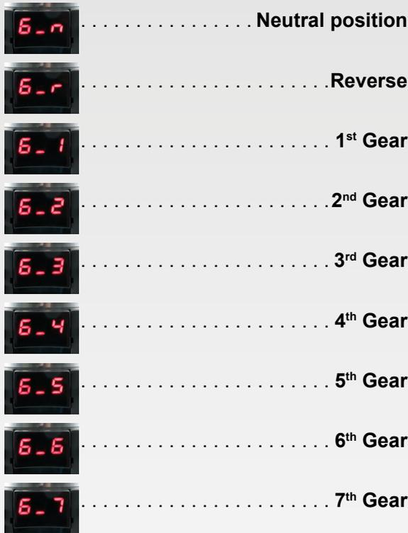
If your shifter has no 7th gear just acknowledge it by pressing
