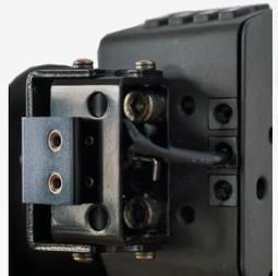
The distance between front side holes and backside holes is 10 mm (centre to centre). The holes have gears for M5 screws. The shifter paddle boxes are already assembled to the Universal Hub for Xbox One out-of-box.
