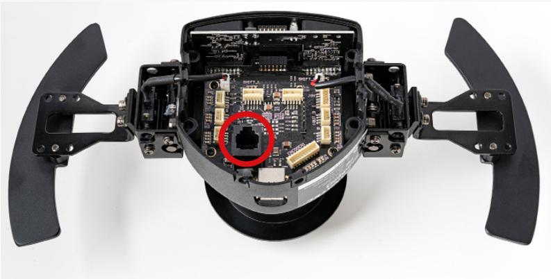
After connecting, position the adapter carefully in a lower hole to prevent damage to the cable.
