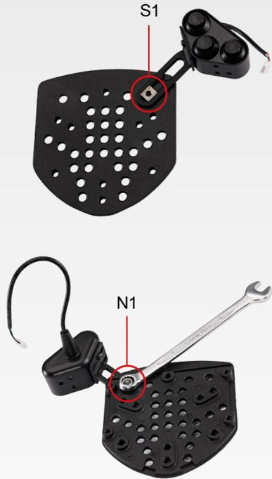
After mechanical adjustment of the FunkySwitch™ you need to make sure that the arrow is located on the top side. If this is not the case you can loosen the small worm bolts and turn the FunkySwitch™. Tighten the worm bolts again after adjusting the arrow position.
