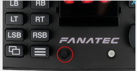
When Tuning Menu is active then press the buttons + at the same time to calibrate the wheel centre.
