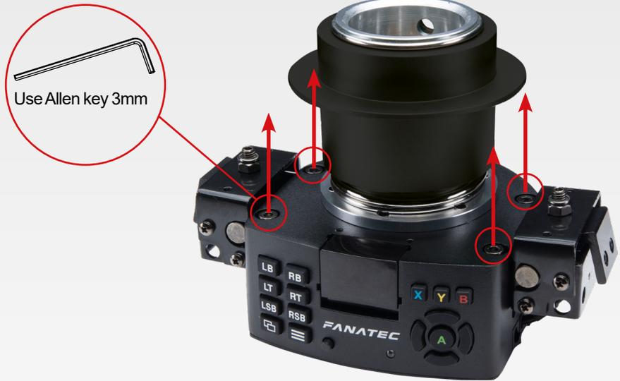
Open the Universal Hub and disconnect the standard shifter paddle cables.
