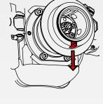
2 Align the wheel base axle to the correct position.
