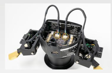
ATTENTION: Position the cables carefully inside the housing to avoid damage!
