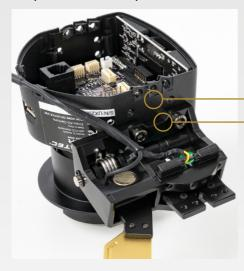
Position 1 - M5x16 mm bolts (I) Position 2 - M5x12 mm bolts (J)
