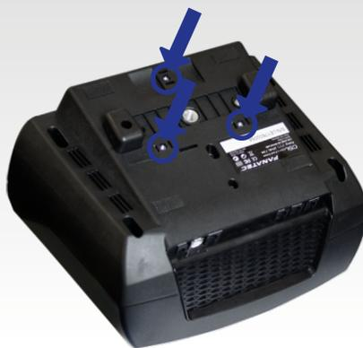
**⚠ IMPORTANT:** Use only good quality M6 bolts. Choose the correct bolt length to prevent the thread from reaching more than 16 mm into the wheel base. **Example: If your table is 20 mm thick, the bolts must not exceed a total thread length of 36 mm!** Always use all three hard-mount points as this allows for a proper and stable installation and avoids damage!
