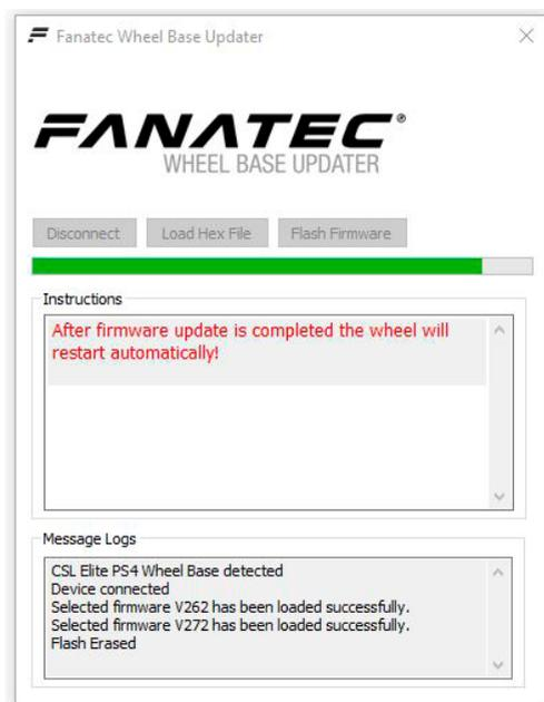
When the update is done the CSL Elite Wheel Base + will restart automatically after firmware update is completely finished as shown on the right-hand side:
