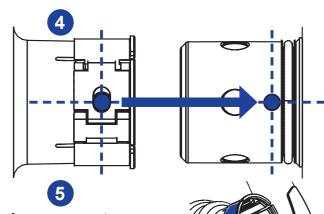
Place and tighten the fixing screw to fix the clamp ring mechanism. Use only the hex key from box contents.
