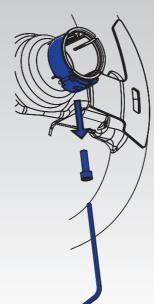
Slide steering wheel off wheel base axle.
