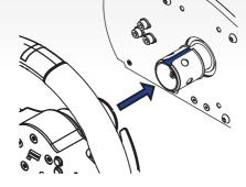
Turn the steering wheel up side down to see the bottom side of the clamp ring to follow next step below.
