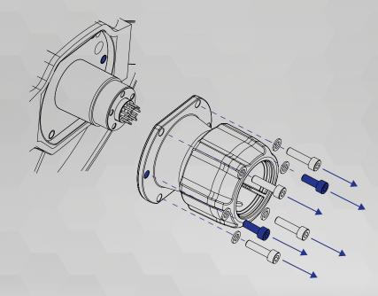
ATTENTION!: Not all bolts are the same length. The two shorter bolts are used on the rounded sides of the ClubSport QRA as illustrated by the highlighted bolts.
