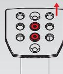
Take off the assembled metal pedal plate and check for the marked holes on throttle pedal arm sides.
