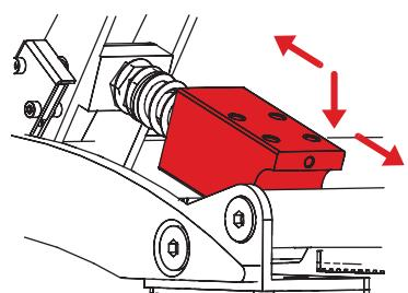
Put the backplate onto the pedalbox again and tighten the two screws with Allen Key 3mm.
