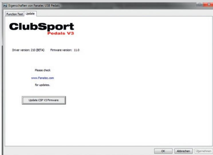
This page gives you detailed information about the currently installed PC driver version and the currently installed ClubSport Pedals V3i firmware version. There is also the button ‘Update CSP V3 Firmware’, see chapter ‘Firmware update procedure’ of this manual for more detailed information about the firmware update process itself.
