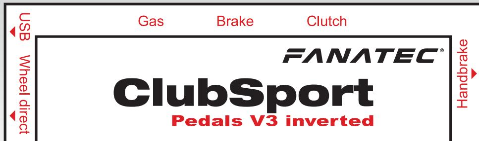
**⚠️ IMPORTANT:** Connect the ClubSport Pedals either by USB cable **OR** by RJ12 cable to a wheel (base). Never connect both ways in parallel to avoid hardware damage!
