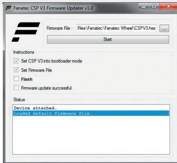
Now the user has the opportunity to select a different ClubSport Pedals V3 firmware file than the default selected file by pressing the button with the three dots if necessary. Usually the latest PC driver version already includes the latest ClubSport Pedals V3 firmware so this step is not necessary for the user.
