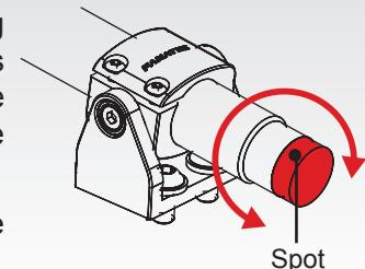
When you have found your favourite adjustment we recommend fixing the knurled plate at damper back end by using the Allen Key 1.5 mm (included in ClubSport Pedals V3i package and ClubSport Pedals V3 Damper Kit package) to avoid maladjustment due to vibrations while driving:
