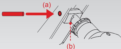
Adjust the preload screw so that the scale is within the correct use range and there is no mechanical play in brake pedal. Note: Preload screw cannot be used in the full range as before, it's use is limited only to eliminate the mechanical play:
