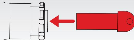
Turn back the brake assembly into the brake pedal lever, then reconnect the loadcell cable to 'Brake' port:
