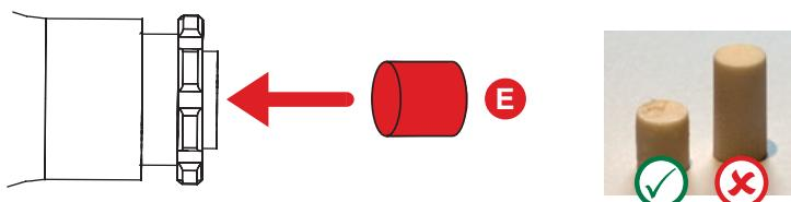
Select two pieces of the Elastomer springs (A) – (D) from Brake Performance Kit package content according to your preferences (refer to chapter 'hardness comparison' of this manual) and apply Lithium grease (F) to their surface:
