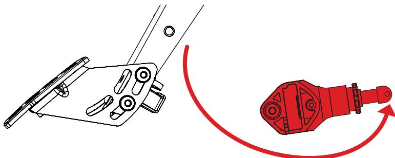
Remove the brake pedal bolt:
