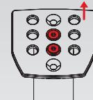
Take off the assembled metal pedal plate and check for the marked holes on throttle pedal arm sides.
