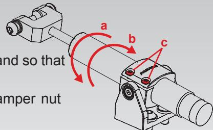
Now you can check the damper effect by pressing the pedal with attached and fixed ClubSport Pedals V3 Damper Kit. At the same time you can change the damper adjustment by turning the knurled plate at the back end of the damper, see picture below:
