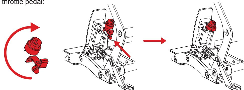
Use the Allen Key 4 mm and screws S2DK with washers W1DK to mount the damper bottom link onto the pedal box (3 screws on brake pedal box, 4 screws on throttle pedal box):
