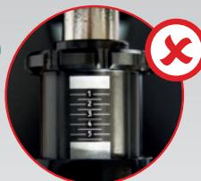
At the brake pedal you can see a dark grey screw with a printed scale. With this screw you can adjust the brake pedal preload (stiffness). Use a setting within the laser scale on this screw: Upper white block has to be completely visible at any time and lower white block never has to be visible!
