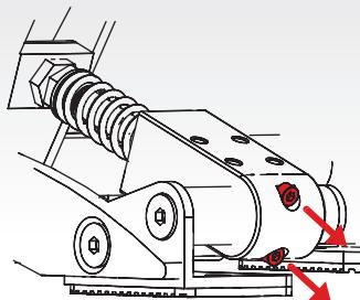
Push the pedalbox towards the pedal lever and away from lower stroke.
