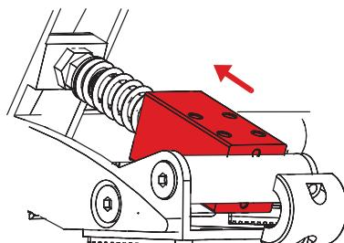
Lift the pedalbox upwards and then pull it from the pedal rod.
