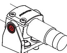
Adjust and lock damper position: Turn the damper backwards until pedal moves a bit (a), then turn damper 180° towards the pedals again (b). Tighten the two screws by hand so that the damper cannot be turned anymore (c).
