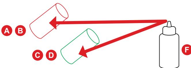
Insert the selected two pieces of the Elastomer springs (A) – (D) into the preload screw:
