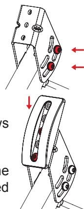
After assembly of the pedal extension at throttle, whether using the metal pedal plate or the D-shaped plate, you need to re-use the distance block and screws to mount the rumble motor again at its original position as shown on picture on the right hand side.
