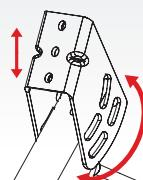
Put the screws S1 into the holes, add a washer W1 and a nut N1 on the back end of the screw S1:
