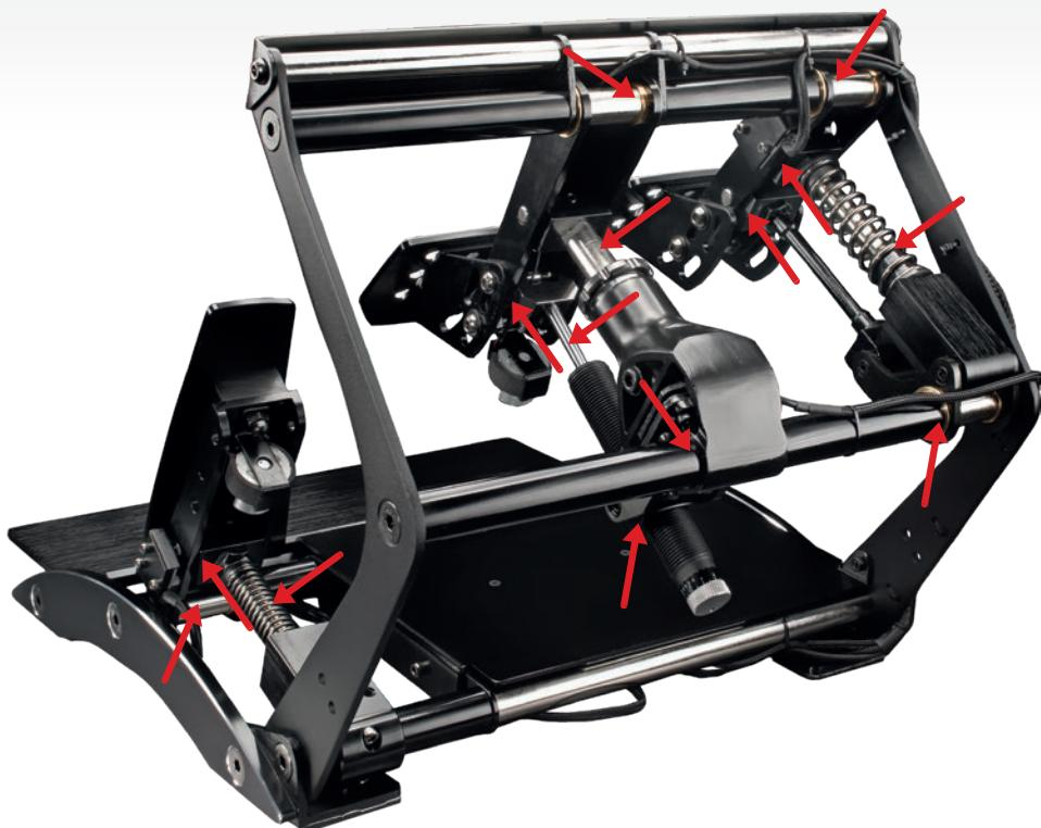
Please add some technical vaseline to the PU foam inside brake pedal if it develops a stuttering feeling. Do **not** use the lithium grease from ClubSport Pedals V3i box content as this might affect the life time of the PU foam.
