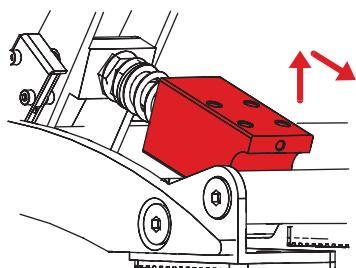
Pull the assembled spring from the pedal rod together with the spring guides.
