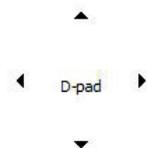
The 'D-pad' arrows (up, down, left, right) change their colour from black to blue when the corresponding direction is pressed on the attached Fanatec Steering Wheel.
