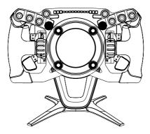
Press the indicated paddle and button combination simultaneously (shown on the next page) to deactivate the illumination.
