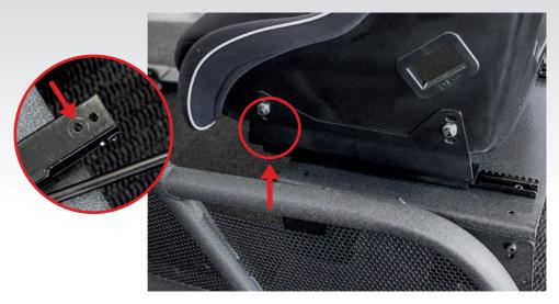
For the last step, adjust the seat fully backwards and mount the two screws in the back:
