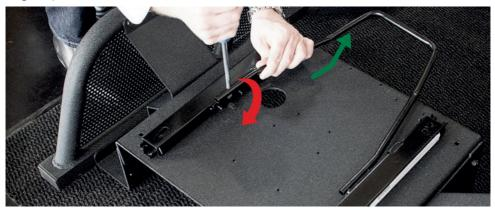
**IMPORTANT:** Make sure that the bar is securely positioned on the posts of the rails as shown below. You might need to use a hammer to get the bar attached on the rails properly.
