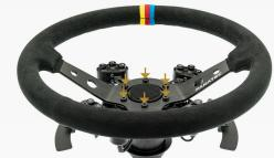
NOTE: Use the bolts included with a max. torque of 2 Nm on your Wheel Rim.
