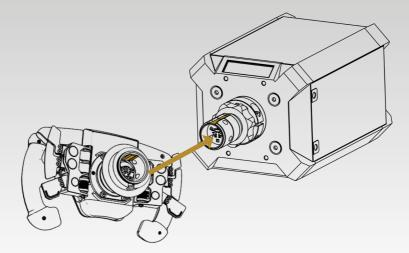
Pull and hold the Quick Release sleeve and carefully push the steering wheel onto the shaft.
