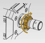
Position the locking ring until it touches the rubber gasket, but do not tighten. This keeps the rubber gasket in place during wheel rim attachment.
