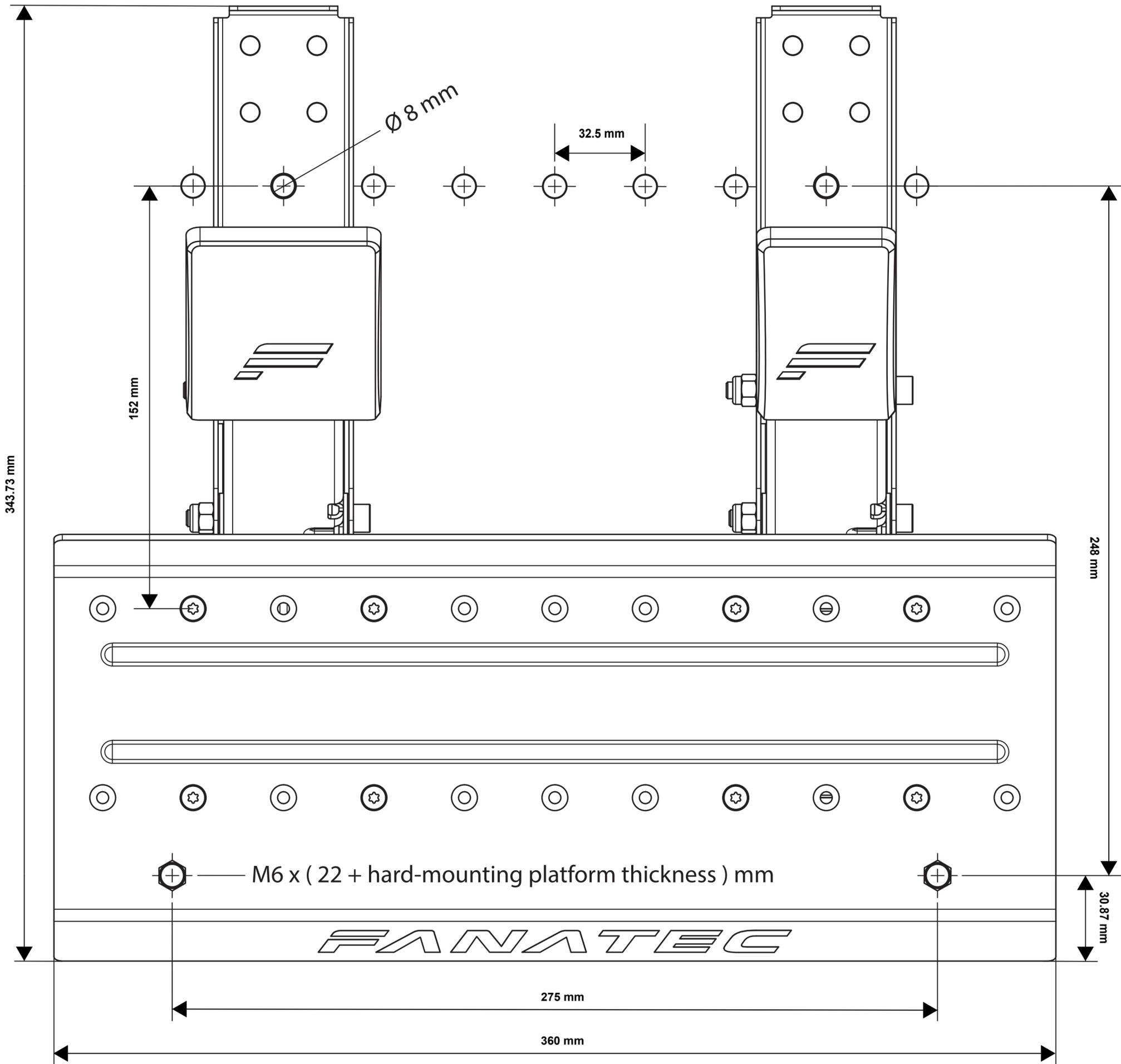
EN: When printing the Drilling Template at home, please make sure that the print size is 100% (file size = print size). Therefore deactivate "automatic page scaling" in the print dialog for example. The overall height of the CSL Pedals is **219 mm**.
